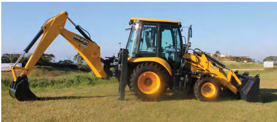
Weighing in at 7 800-8 750 kg, the 883 Dezzi CMI is fitted with a standard 1,1 m 3 bucket.
