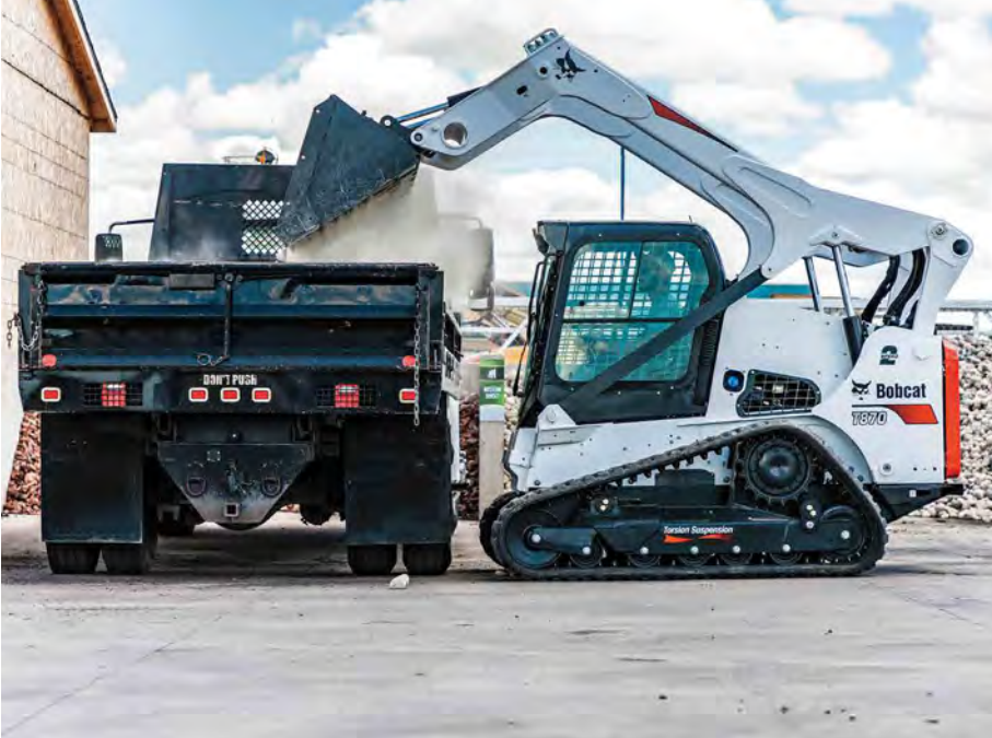
Bobcat's new T870 torsion suspension machine offers 10% more lift capacity than the previous roller suspension model.
