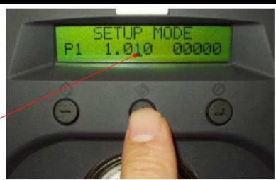
5. Press and hold Set Button for 2 seconds to save data
