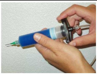
5. Connect plug end of Receiver Head Assembly to air outlet
