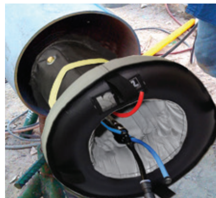
QuickPurge features an additional gas input line
