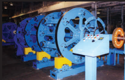
▲ 24 wire planetary strander recently shipped to China
