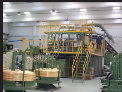
▲ RS 2500 machine casting 8mm diameter brass wire rod
