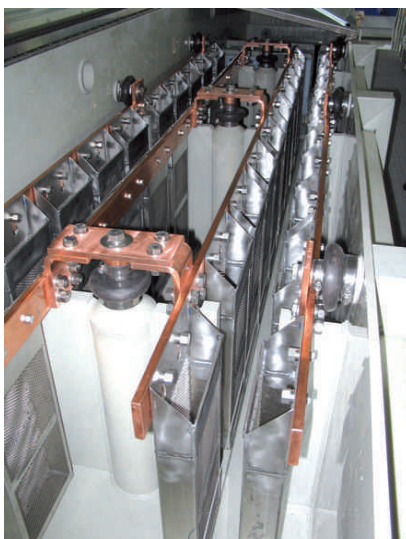
▲ Anode basket with anode material
