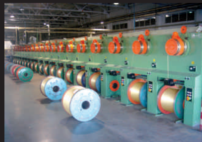
▲ Spool take-up frame with double accumulation capstan for non-stop operation
