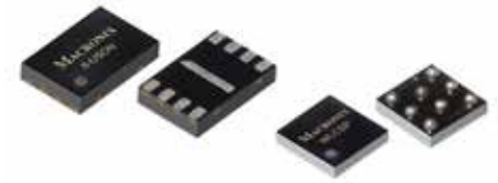
Fig 2: USON and WLCSP packages for the Macronix Serial NOR Flash MC25R Series
