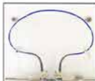
Flex Test™ setup shows triple strain relief, effective through 20,000 flex cycles for all models.
