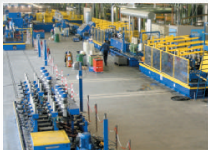
Tube mill for production of stainless steel H.F. welded exhaust tubes - max. production speed 120 m/min
