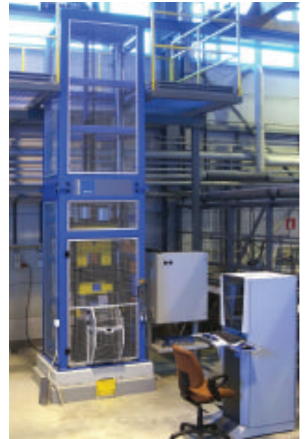
Drop weight tear tester with 25,000 joule capacity
