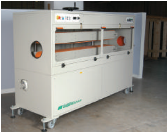
⚠ Gillard's new machine has longer belts for less pressure on extrusions
