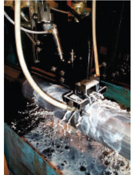
Based on phased array technology, the weld profile visualization system is used for scarf monitoring
