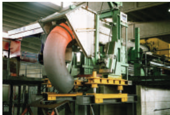
Fabrication of a 24" pipe bend with inductive heating
