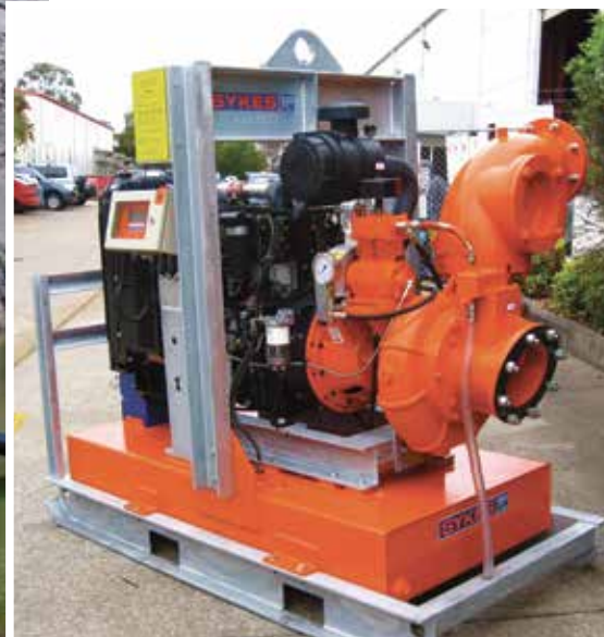
The Sykes Contractor pump is a true self-priming pump, and does not require manual priming of a suction line or filling of a priming tank to begin its normal operation.
