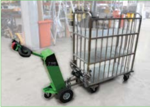
Shown with electric clamping hitch
