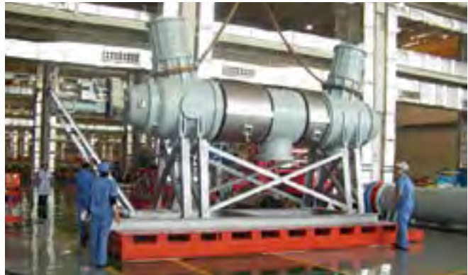
Large platform with bearers to aid forklift loading
