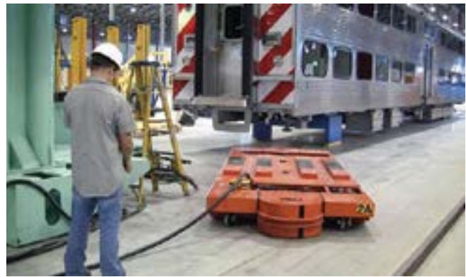
Air skid with guide wheels for direction control
