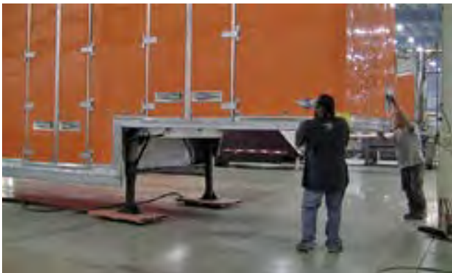
Multiple air skids to allow movement of semi-trailers
