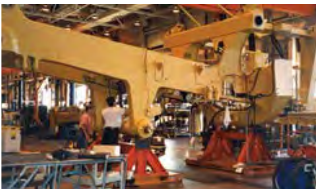
Multiple air skids to allow movement of an awkward and heavy item
