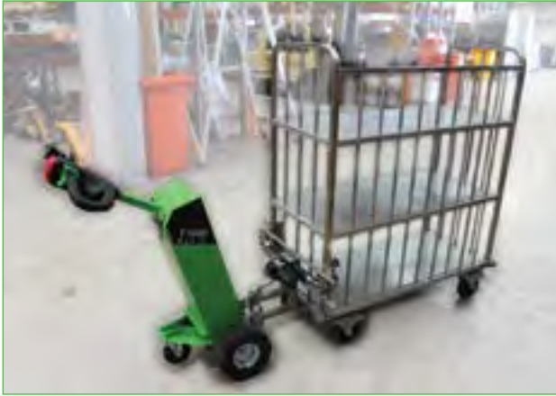
Shown with electric clamping hitch
