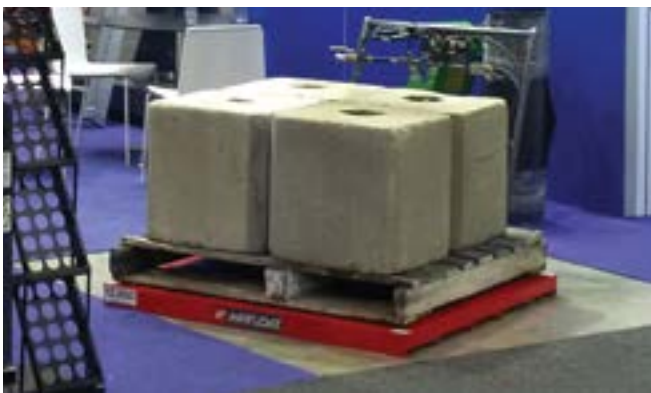
Pallet sized air skid with push handle
