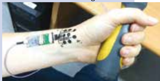
Temporary-tattoo for long-term high fidelity biopotential recordings.
