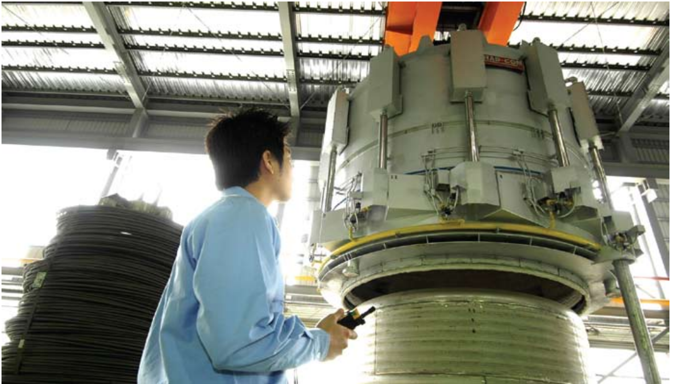
▲ Rad-Con's 100% hydrogen super-high convection bell-type annealing furnace
