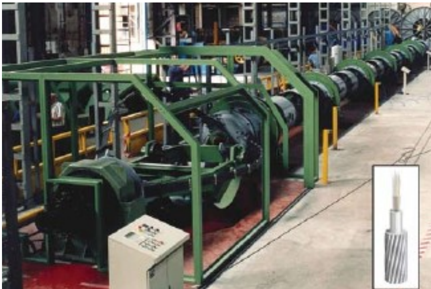
▲ Tubular bullhead strander for OPGW
