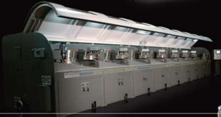
Cold rolling lines with cassettes
