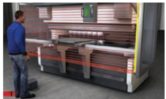
The SPG system reduces installation and service costs because there is no set-up or alignment of muting sensors.
