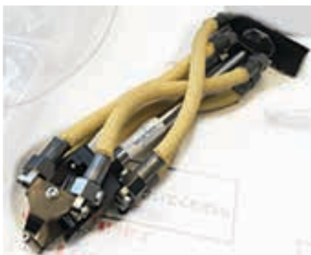
Figure 4: Application to the robot arm. Right: two robotic arms using the artificial muscle. Below: A wrist of a robot with six artificial muscles.
