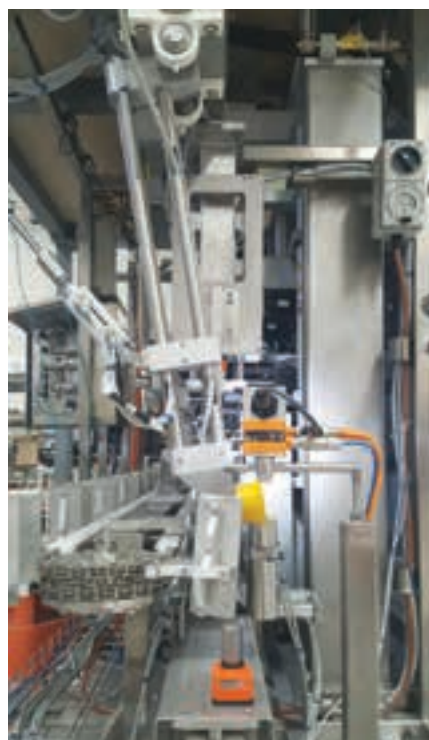
Using a servo-controlled indexing system and a verification sensor, the carton erector places and orients the carton for filling.
