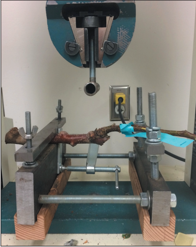
Fig. 1: Apparatus used for 3-point flexural strength testing. Sample supported with 16 cm separation with flexural strength and rigidity measured with a bench-testing machine. The sample shown is in "bud up" position where the chip bud is situated proximal to the displacement force.
