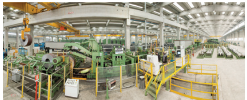
Figure 1: Strip preparation and spiral strip accumulator
