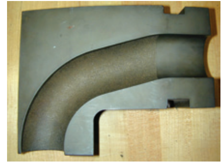
Bending die with Carbinite coating
