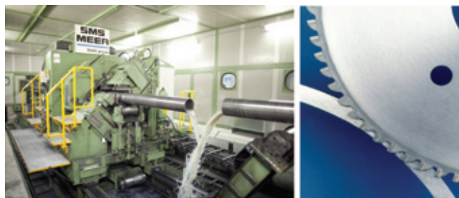
Figure 8: Travelling milling cut-off unit with milling cutter blade
