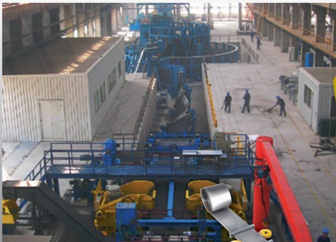
Strip edge milling machine BFMK for welding edge preparation with highest accuracy
