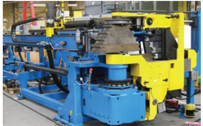
An AddisonMckee DB 89 electric bending machine
