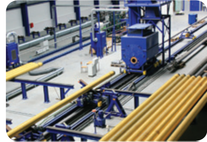
Internal blasting & lining
