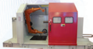
HD-1630/800/1000/1250/1400/1600/1800/2000mm PLC High speed cantilever type single twister (cabler)
