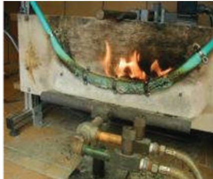
○ Picture 2: IEC 60331-25 fire test
