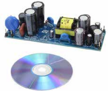
Figure 4: STMicroelectronics power supply reference design for smart-metering applications.
