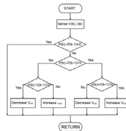
Figure 3a: The basic P&O algorithm (Source: MATHWORKS)
