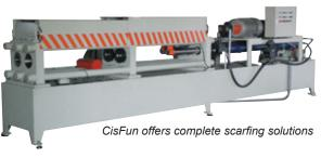
Some of the features include: mechanical inside tube scarfing tools and feeding by hydraulic system with a tube ID range of 12mm – 200mm. They are suitable for a maximum tube length (auto feeder) of 6m but special
