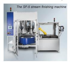
whilst the process is running, making down time for loading and unloading unnecessary. The machine has five grippers that can hold items such as thread taps or carbide drills of widely varying diameters: two with diameters of over 10mm and three with diameters of less than 10mm. Workpieces with diameters ranging from 2 to 20mm and with lengths of up to 350mm can be inserted.
