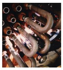
The OP heads are suitable for producing pipe coils for heat exchangers, collectors and in boiler construction
