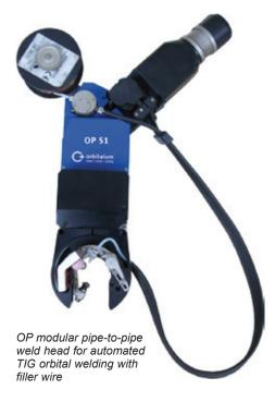
pipe diameter of 25.4mm. With the large OP 102 version for pipes up to 102mm in diameter (diameter of the head module of 190mm), a pipe gap of 46.2mm is sufficient for a 101.6mm pipe.
