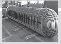
**Grades:** Austenitic (304,310, 316, 321 etc.) Duplex (2101, 2205, 2304, 2507) **Specifications:** ASTM/ASME A/SA 213, 249, 269, 312, 358, 789, 790, 928, API 5LC
