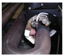
With the smallest version, the design engineer can set the gap between the pipes to just 31.8mm with a pipe bundle having a pipe diameter of 25.4mm
