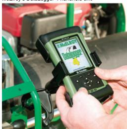
The DataLogger 4 has a wide range of enhancements over previous models. One of the major additions is FusionGuide™, a feature designed to give a faster visual 'go/no-go' interpretation of the graphs presented on the handheld computer and the PC after data download. A trained inspector could look at the generated graphs and determine if a fusion joint was fused with the correct pressures and times according to published standards.
