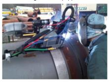
high-speed return feature for faster repositioning of the carriage.
