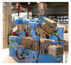
due to the unique "piggyback" system, shortage of space at the plant was no longer an obstacle. The guaranteed output with the CON 50 conical extruder as coextruder is for PVC window profiles 125kg/h and for rigid-PVC profiles 150kg/h. To increase output, High Tech Extrusion is now working on a solution for the conical extruder CON 63 as coextruder. In this case a successful mounting is dependent on the size of the main extruder.
