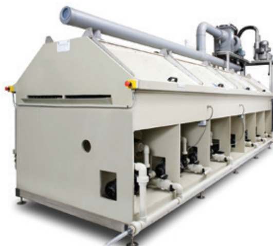
▲ The multi-wire ultrasonic cleaning plant for removal of calcium and sodium wire lubricants
