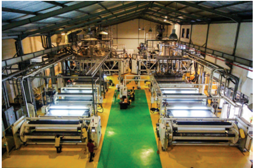
▲ PT Kencar Sukses Investama is expanding its presence in the Southeast Asian film market by adding two more Davis-Standard cast film machines
