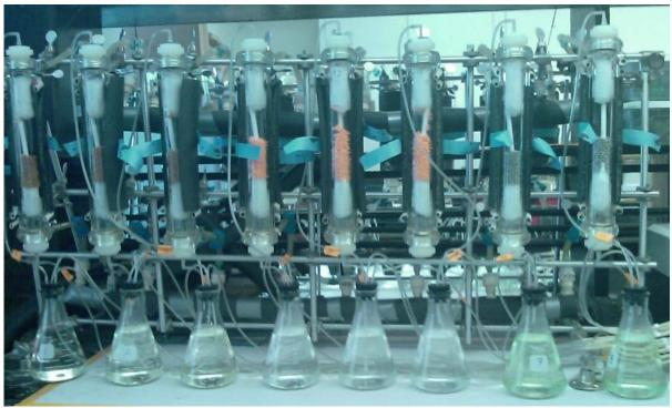
Figure 2015.15C. Extraction apparatus with eight jacketed chromatography columns.
