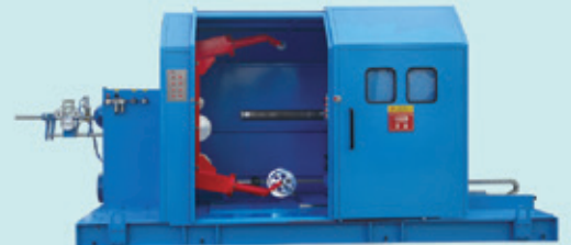
XBΦ500-Φ2500 Cantilever type single twisting machine
