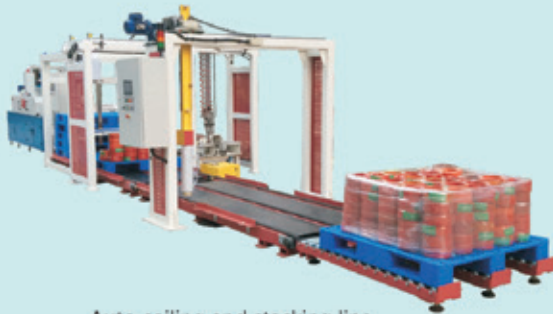
Auto coiling and stacking line
