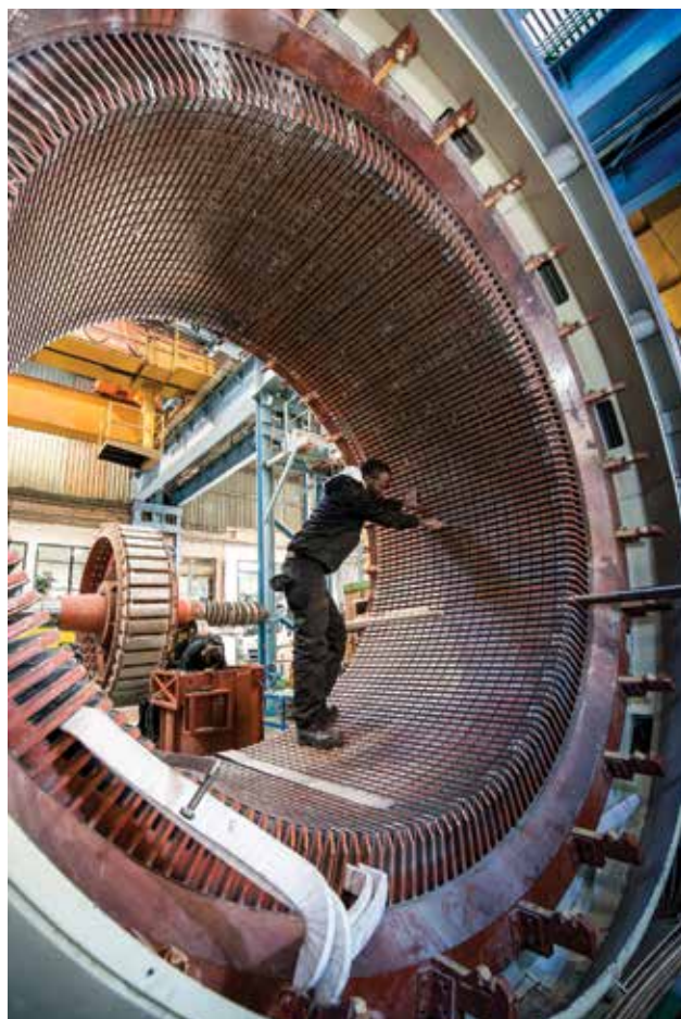
The 65 ton stator mass driving a squirrel cage induction motor very probably makes this the largest motor of its type in the world.
