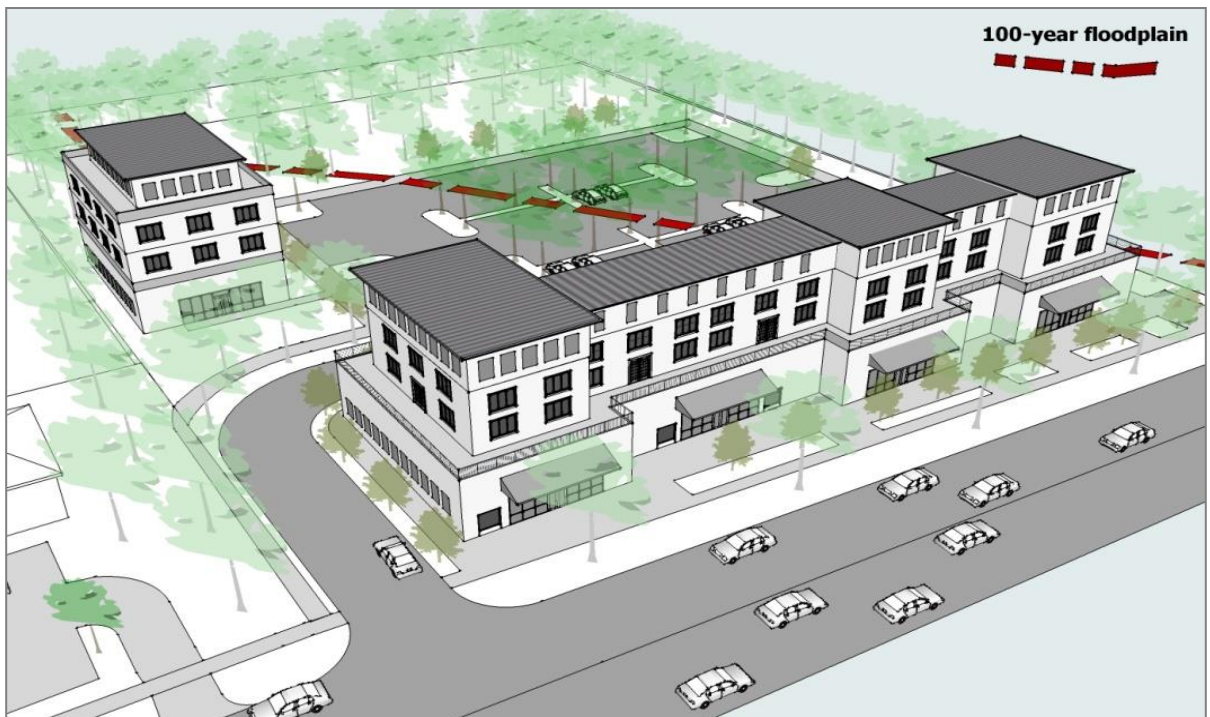
Figure 3.6.3.B: Maximum Structure Height in Relationship to Floodplain Location
