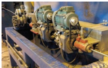
▲ Rod cleaning and wire drawing by DCCD process
