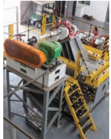
To ensure that the vibrations do not carry into Kwatani's test building, the rig is placed on a secure sub-frame to dampen the movement and dynamics to the floor.
