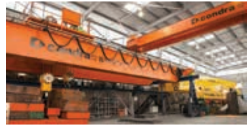
One of the three cranes for Grootegeluk undergoing load testing at Condra's Germiston factory.
