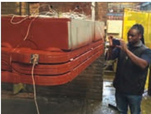
Marthinusen & Coutts' David Motloung records photographic evidence of tests on one of the enormous gearless mill drive rotor poles recently refurbished by the company.
