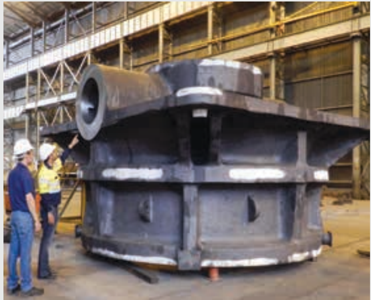
One of the largest spares to be ordered from and manufactured by TAKRAF Africa – a top and bottom shell for a 60/109 primary gyratory crusher for Sishen.
