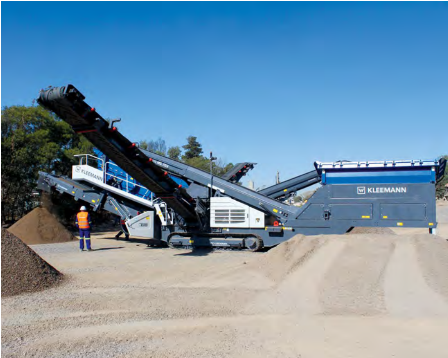
The Mobiscreen MS 703 EVO is a triple-deck mobile classification screening plant for screening all types of stone of up to 150 mm, up to four fractions.
