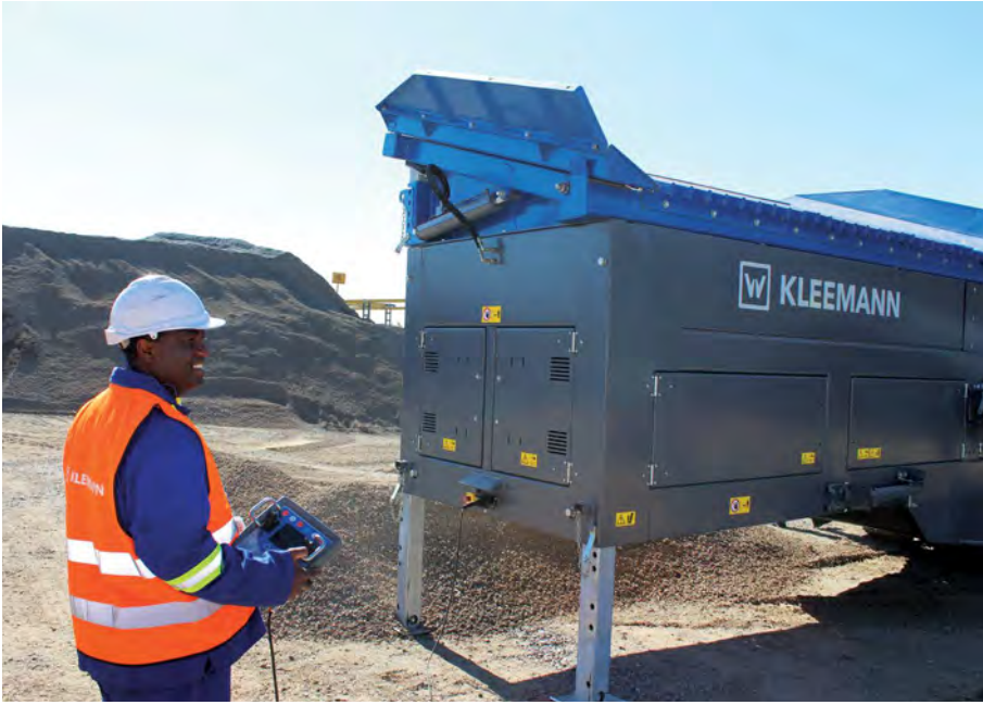
With safety in mind, the MS 703 EVO screen comes with a very big safety feature of being able to unfold the entire machine via remote control.
