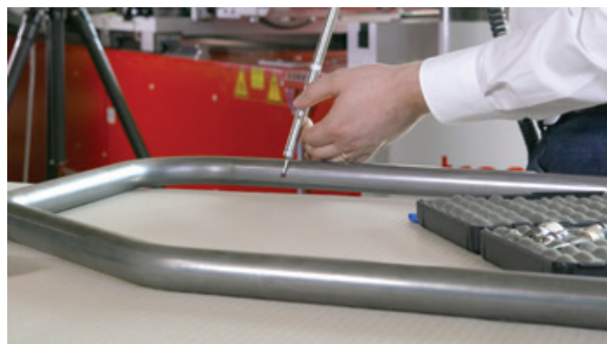
The wireless t control system can be used to measure tubes and connection elements like flanges directly on site
