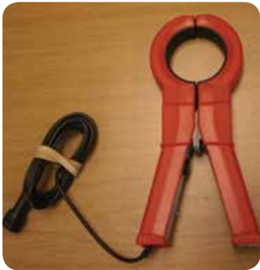
The Universal Technic current probe model SC 2000 has a capability of measuring ac/dc current up to 2 000 A and the frequency range is from dc to 10 kHz with an accuracy on dc of ± 1% and ac accuracy at 50Hz of ±0.5%. The model in the above photograph has a 52 mm jaw and a co-axial cable terminated with a BNC connector. Other jaw sizes and current ratings up to 7 500 A are available from Denver Technical Products.
