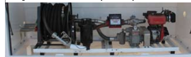
Custom built hydrant cart incorporates filtration with pressure differential gauge, NMI certifiable flowmeter, hose reel & delivery hose with nozzle, hydrant connection hose with drybreak fittings. Also included are spill kit, static reel & fire extinguisher. The unit is easily manually maneuvered to where required.
