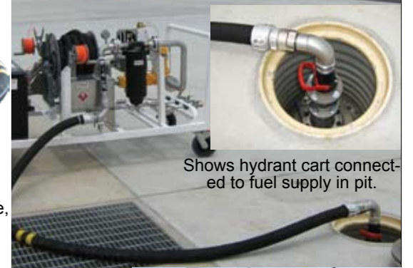
Emergency engine-powered backup pump system
