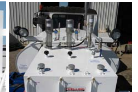
Multi-compartment oil tanks
