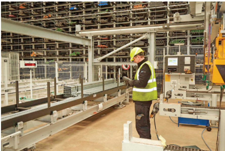
One of the input/output stations serving the KASTOunicompact warehouse
