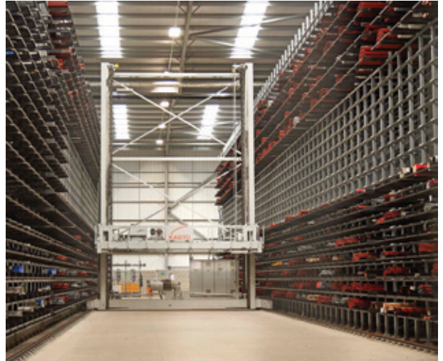
A view of the KASTOunicompact 4.0 automated warehouse for pipe and other materials at the Measham distribution centre
