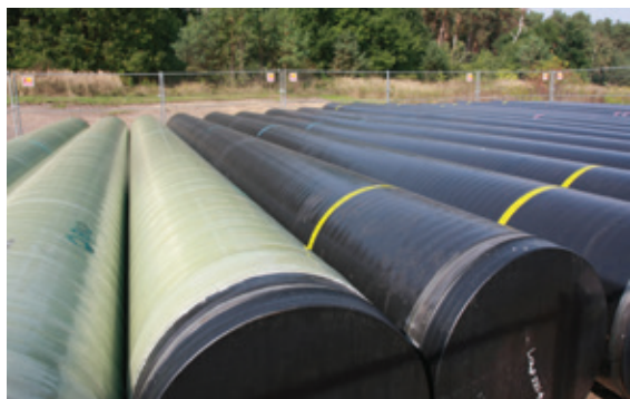
Gas pipes with (left) and without BWB surface protection
