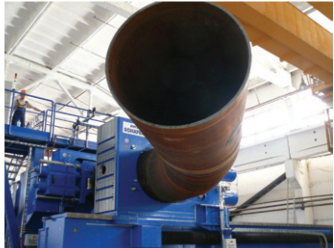
Figure 1: With induction bending machines such as this SRBMI with a feedrate force of 2,000kN, AWS Schäfer Technologie GmbH has become the world leader in recent years
