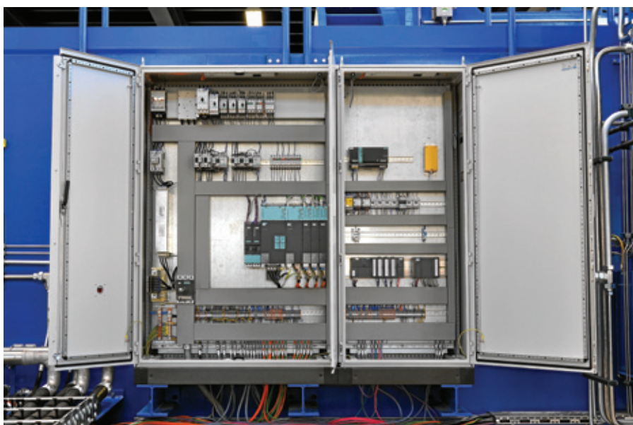
Figure 3: A Simatic 317T Technology CPU from Siemens maintains the constant velocity of the hydraulic feed axis and perfect coordination with further servo axes – ensuring a constantly high and reproducible bending quality
