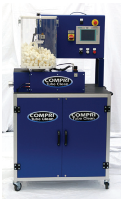
Bison W/D uses both dry and liquid-soaked projectiles
