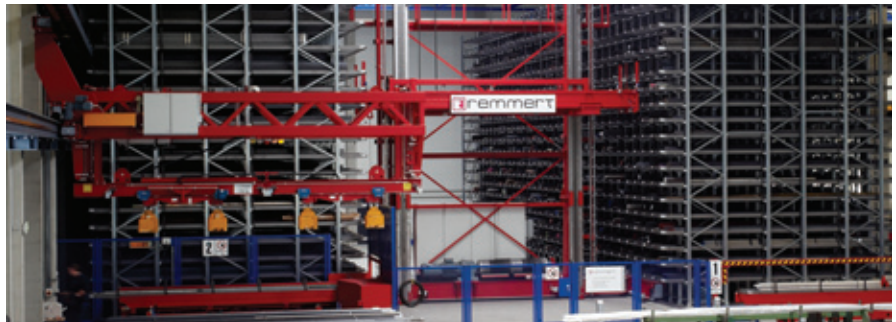
The Remmert honeycomb storage system
