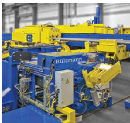
Drawing steel tube up to 150mm diameter
