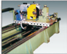
Burr free cold saw fly cut off
