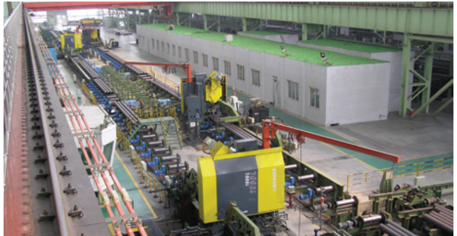
KSA 1600 L cold circular sawing machine for seamless steel tube production
