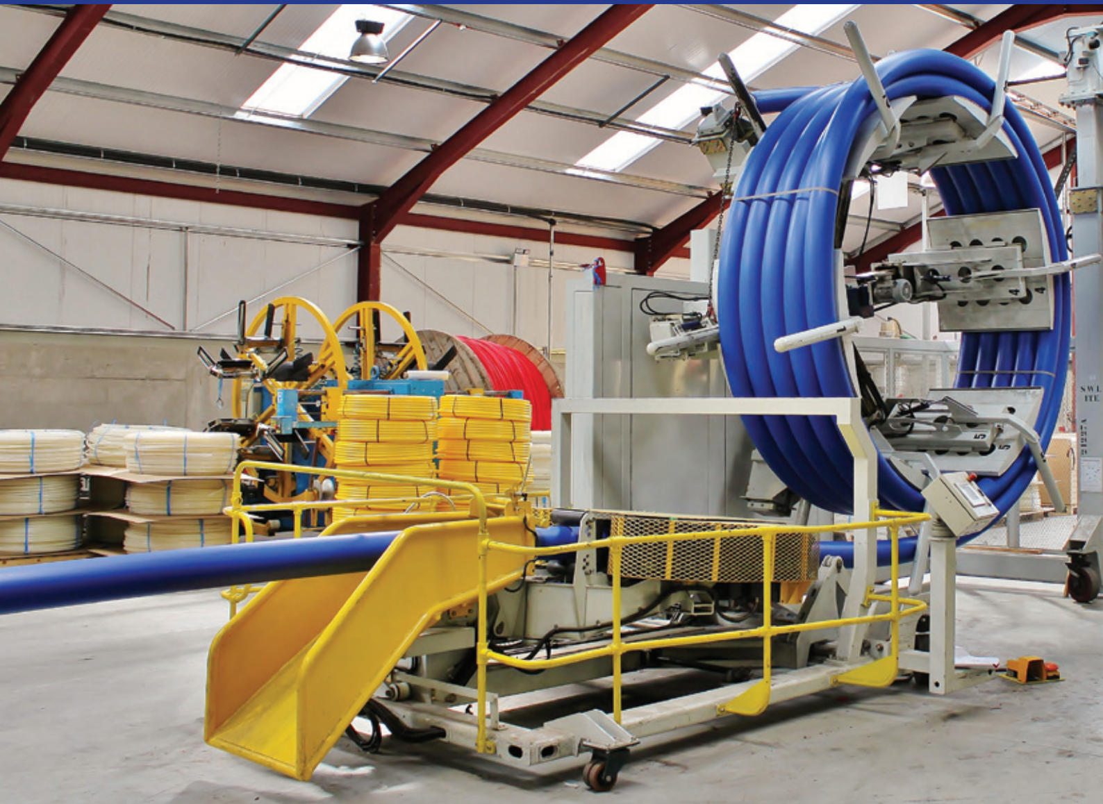
Pipe Coil Technology Limited: The Low Ovality technology in action (see page 217)
