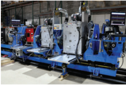
Multiple test Echomac ultrasonic and Rotoflux transverse and longitudinal flux leakage system to inspect steel tube
