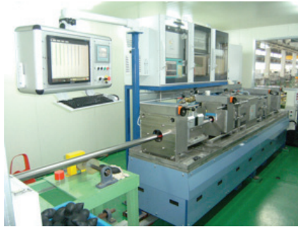
RotoUTscan for titanium tube inspection up to 65mm
