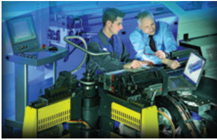
Tubotron Vario 40 RL all-electric right- and left-hand CNC tube bending machine for complex tube shapes
