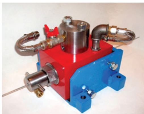
▲ Wire cleaning by PWC-S system
