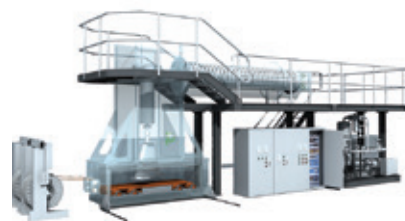
▲ IBA's Easy-e-Beam®: An integrated crosslinking solution including a self-shielded E-beam accelerator, pay-off, take-up and the overall control system
