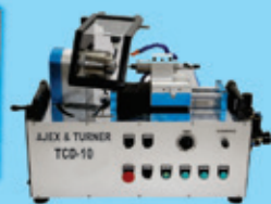
In-House Pneumatic Carbide Die Polishing Machine
