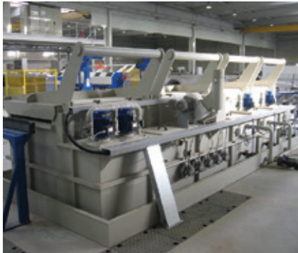
▲ Ultrasonic and electrolytic cleaning from Sirio
