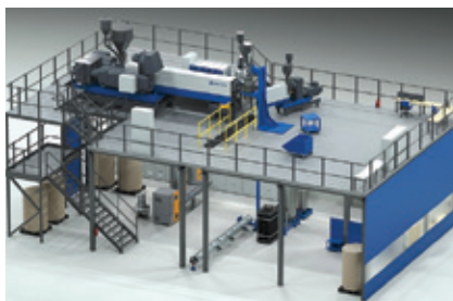
▲ A pilot-scale vertical extrusion group for medium and high voltage cable production in Maillefer's R&D centre in Finland
