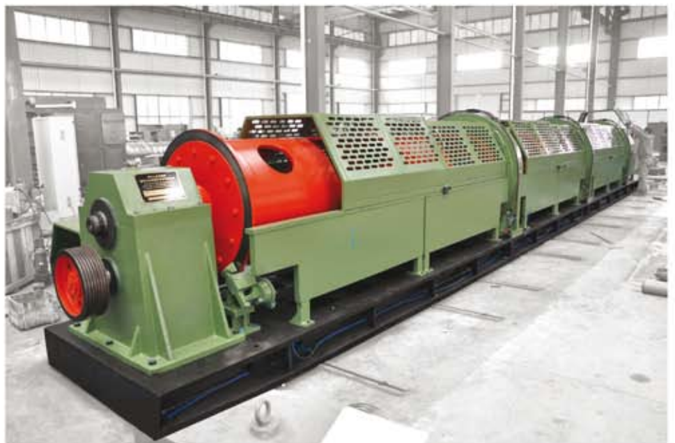
High Speed Tubular Strander Type JG630/6 with Large Bearings
