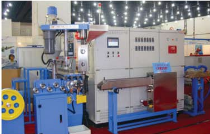
UL電子線生產線 光伏電纜生產線 電纜纜生產線 PU生產線 高密度、低密度生產線 BV、BVR生產線 彩帶挤出機生產線 電源線、尼龍線、建築線、低低煙油、絕緣護套生產線 Ø30mm-Ø120mm高速電纜電纜擠出機系列(全程PLC人機界面控制) Production line for telephone line,PU production line, high-density and low-density production line, BV, BVR production line, Extrusion production line of the colored lights Production line for power cable, Nylon line, building line Low smoke halogen free cable, insulation sheath High speed wire and cable extruder series (full PLC man-machine interface control)
