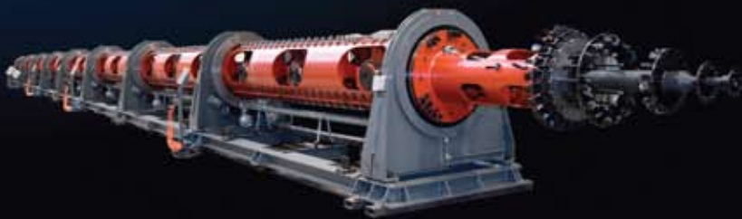
Tubular strander for copper, aluminium or steel wires
