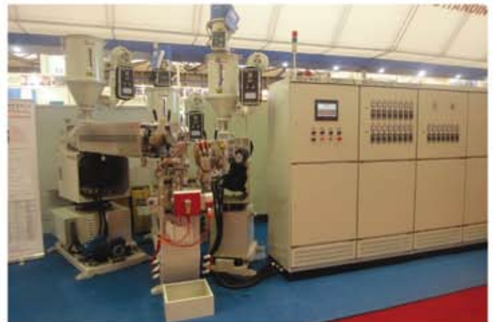
HD-Ø70+70+50mm PLC 高精度三層共擠擠出機 HD-Ø70+70+50mm PLC High precision three layers co-extrusion extruder 最新瑞士機型 The latest Switzerland type
