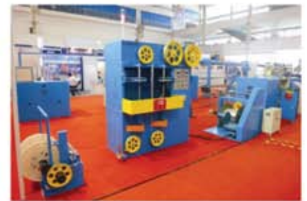
HD-Ø630/800mm 單層雙層三層繞包機 HD-Ø630/800mm Single layer, two layers and three layers wrapping machine (for mica, aluminum foil) 最新機型 The latest type
