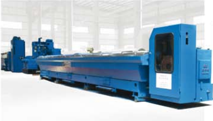
Copper Wire Drawing Machine Type LHD 450 Series (With Continuous Annealer and Quick Die-change)
