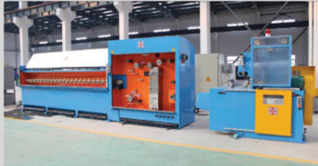
Multi-wire drawing machine with continuous annealer
