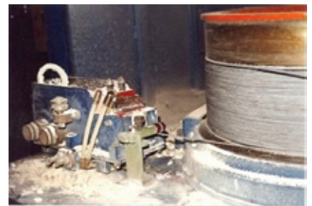
▲ Rod dry coating by LVC/PDH system, in a 0.85% application
