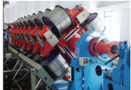
Rigid Wire Stranding Machine with Auto Batch Loading System
