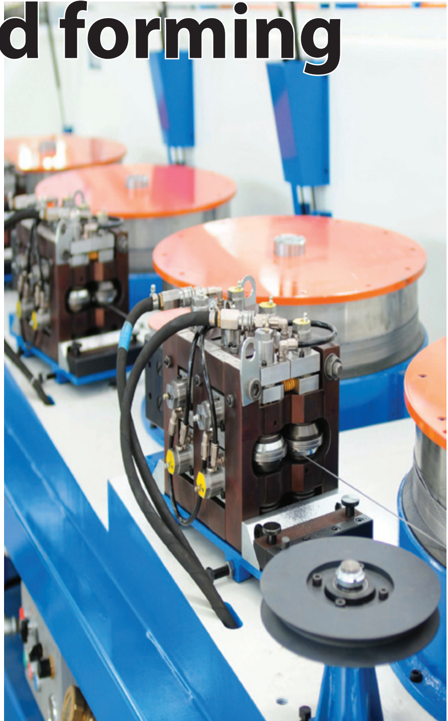
▲ Drawing line converted from die to micro-rolling concept
