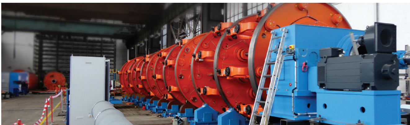
▲ Sket's tandem cage type stranding machine was delivered to a Scandinavian company
