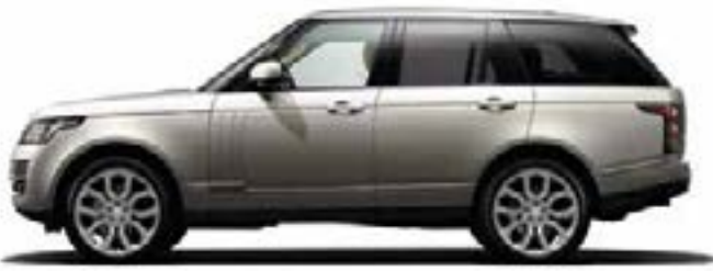
Standard Wheelbase (SWB) 2,922mm
