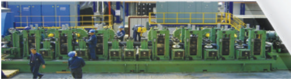
ERW TUBE MILL 1/2"-24" (API/ASTM)
