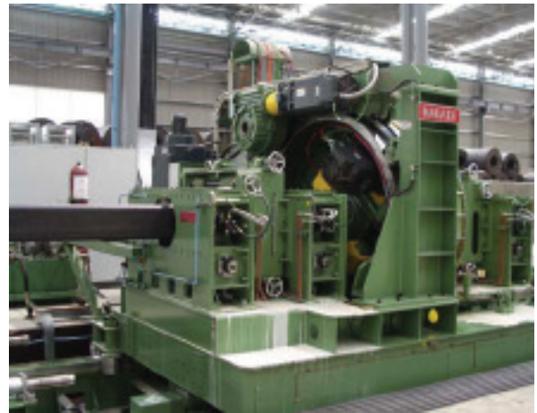
12" Milling type flying cutoff machine
