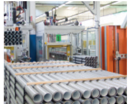
The Multipack and Multipallet machines are designed for packing rigid pipes
