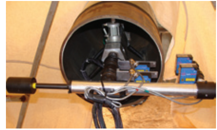
The Model 224B Bevelmaster ® as the primary weld prep tool for a special land-based pipeline with Inconel lined bore
