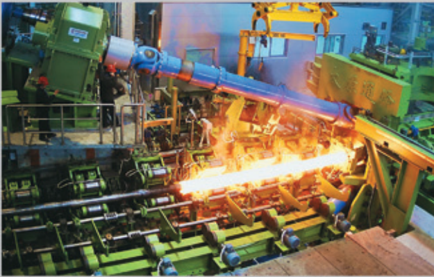
New cone type piercer for TPCO 258 line
