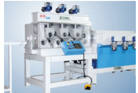
MRP60D straightening machine for complex profiles
