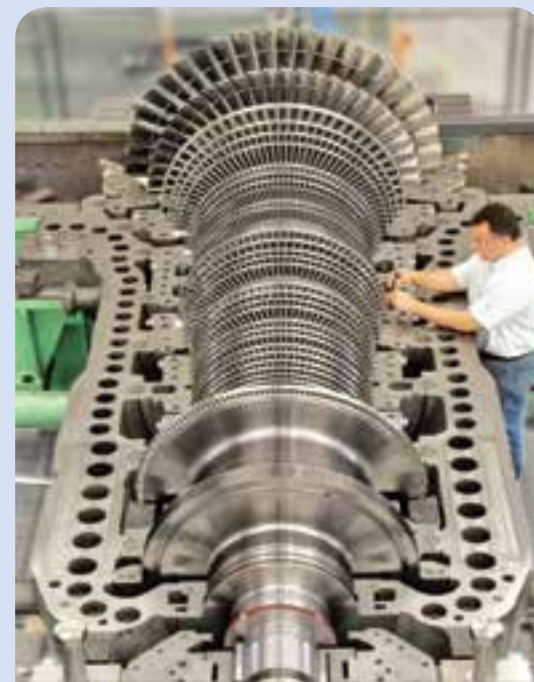
The 48 MW TGM multi-extraction condensing steam turbine rotor, which is designed to maximise efficiency and power generation capability.
