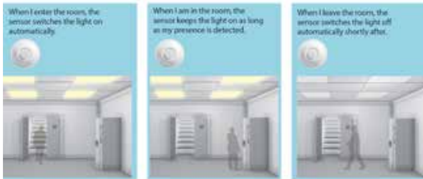
The Legrand PIR ceiling mounted lighting management sensor, with 180° infrared detection, is ideal for passageways
