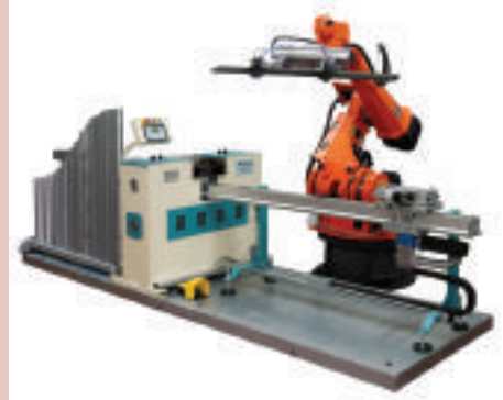
↑ The new robot transfers workpieces to Apollo's Twin punching lines
