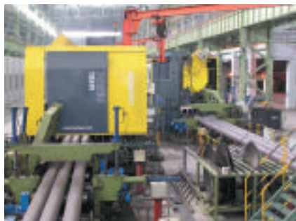
Linsinger's KSA 1600 carbide circular saw
