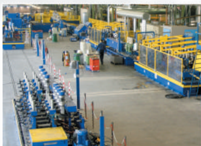
Tube mill for production of stainless steel H.F. welded exhaust tubes - max. production speed 120 m/min
