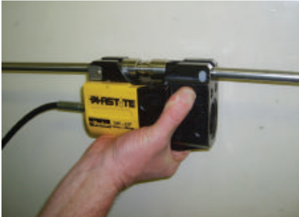
Phastite tooling allows assembly directly against panels and bulkheads
