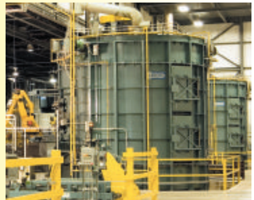
A Can-Eng basketless heat treatment system
