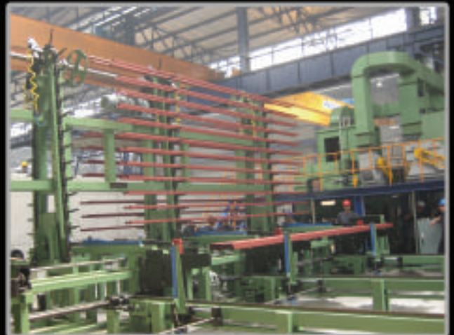
Factory space save by tube dry elevator
