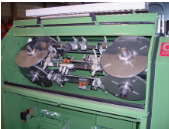
▲ The new high-speed 8-pad taping head
