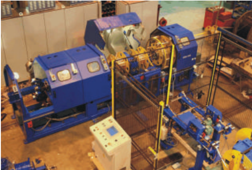
▲ Pourtier CAH 670: double head version for 2 strips
