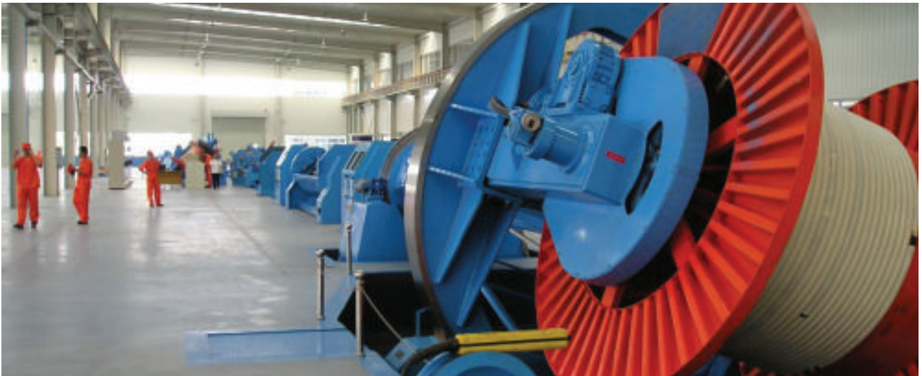
▲ Gauder's latest drum twister, the largest of its type, will be supplied to Saudi Cable Company
