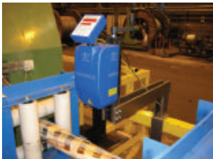
▲ Proton's IntelliSENS for cable measurement!
