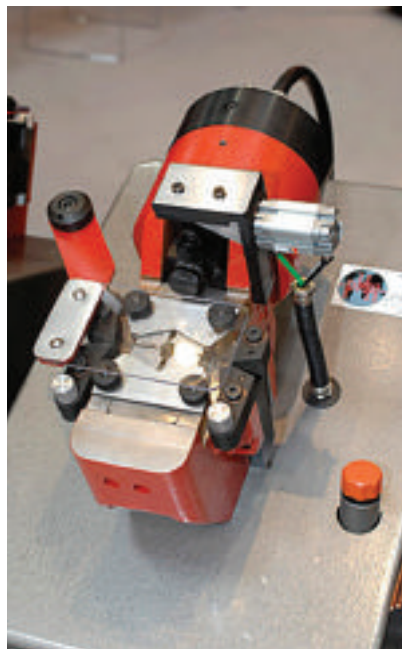
▲ The welding head of the new HP100 auto air/hydraulic cold welder
