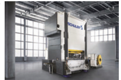
▲ The Smartline from Schuler for the interlocking of electric motor laminations machines a blank thickness of 0.2mm. Photograph courtesy of Schuler
