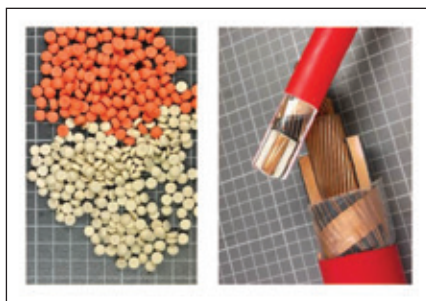
▲ Figure 1: MV insulation containing lead (orange) and lead-free (white), from pellets to cables
