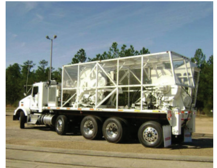
Cable pulling unit for WA Chester LLC
