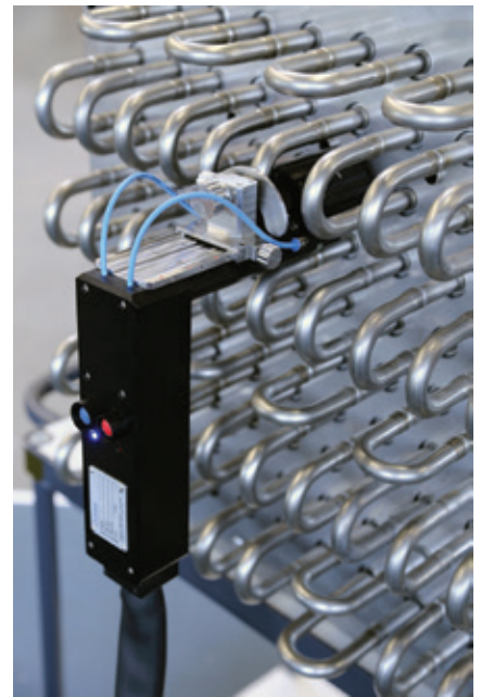
The HX 16P features pneumatic clamping of the head
