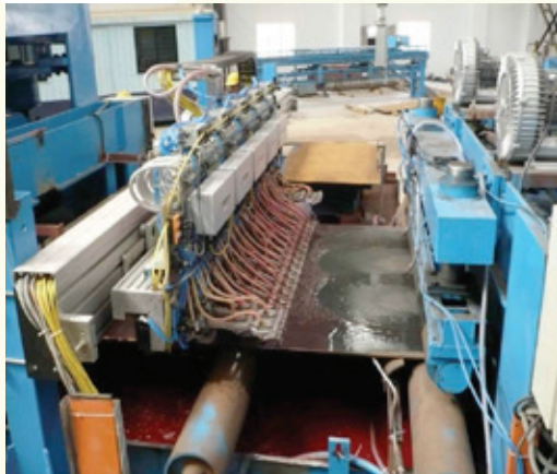
Spiral mill 2 m coil - Thickness 5 – 25 mm
