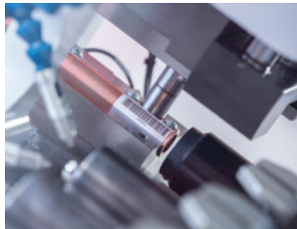
Prior to end forming, the operation parameters are read via a barcode
