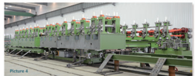
Picture 4 Changing base for offline automatic roll change, size changed in 30 minutes
