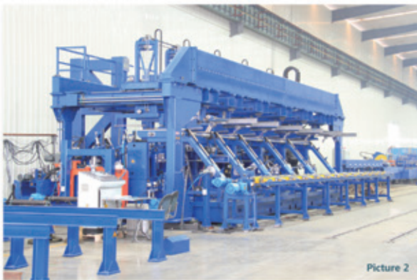
Picture 2 Automatically rapid packing machine with water dumping, pipe bundle weighing and stacking
