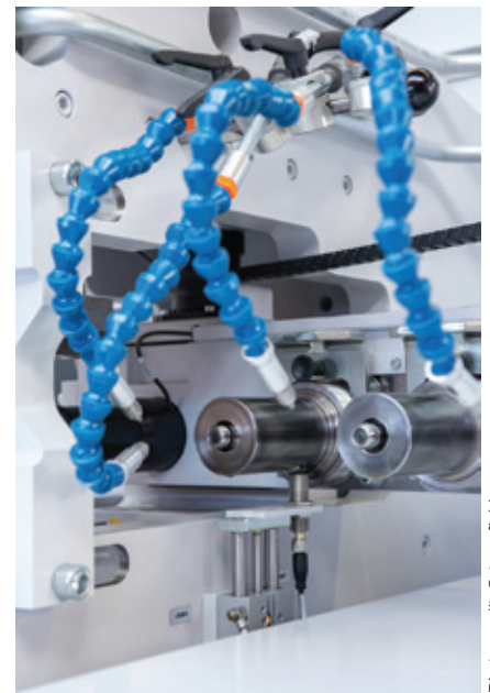
All tools of the REB 645 are equipped with RFID sensors
