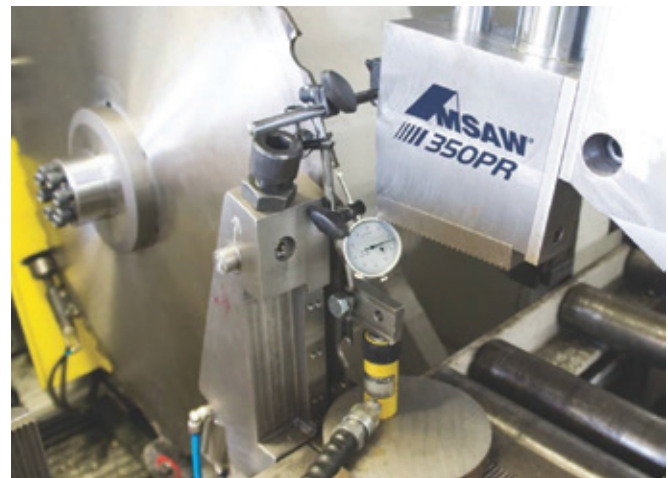
Figure 2: Hydraulic cylinder applied tangential force on the blade and the displacement was measured with a dial indicator
