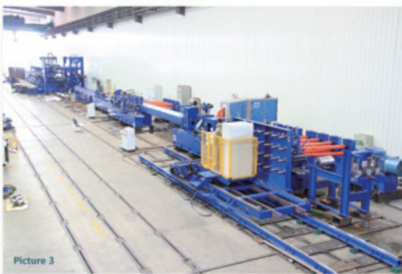
Picture 3 Automatic roll change robot for \phi 127 mm pipe mill with inline automatic roll change and adjustment, size changed in 60 minutes
