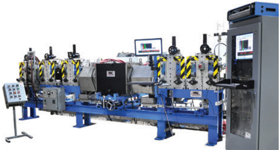
The multi-test system for automotive shock absorber tubing and OCTG features 100mm ultrasonic Echomac rotary test and a MultiMac eddy current tester
