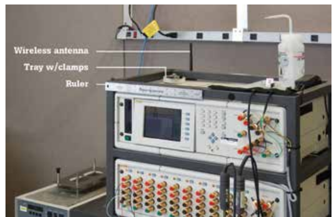
Figure 5: A wireless modem and frequently used tools like rulers and clamps were placed on test stations for significant time savings.
