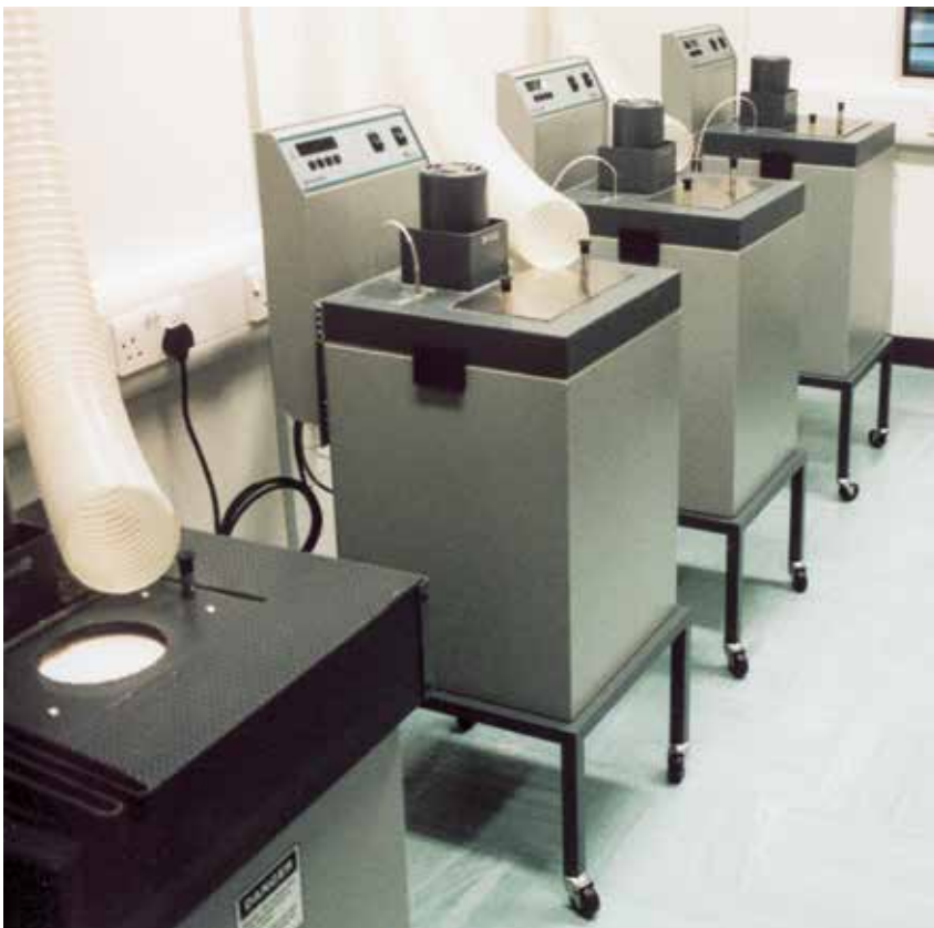
Figure 1: Full-sized stirred-liquid calibration baths used in a PRT Calibration process.
