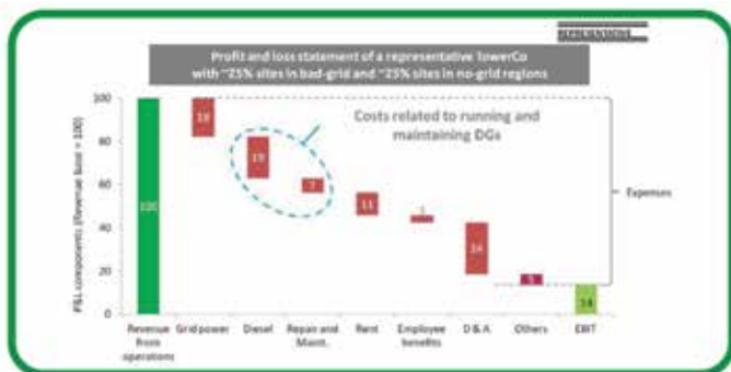
Figure 1: Operating diesel generators in regions with unreliable or non-existent power grids account for over 20% of a company's expenses.
