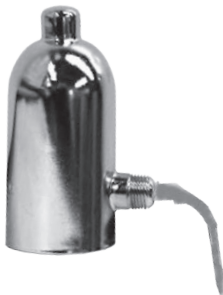
STEAM AIR VALVE DOLE SERIES 1933 • 1/8" NPT This low-cost valve is for venting radiators of hand-fired systems. Large float provides a seal against condensation to stop spitting.
