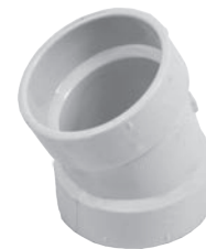
22° ELBOW • PVC-DWV (HUB x HUB, 1/16" BEND)
