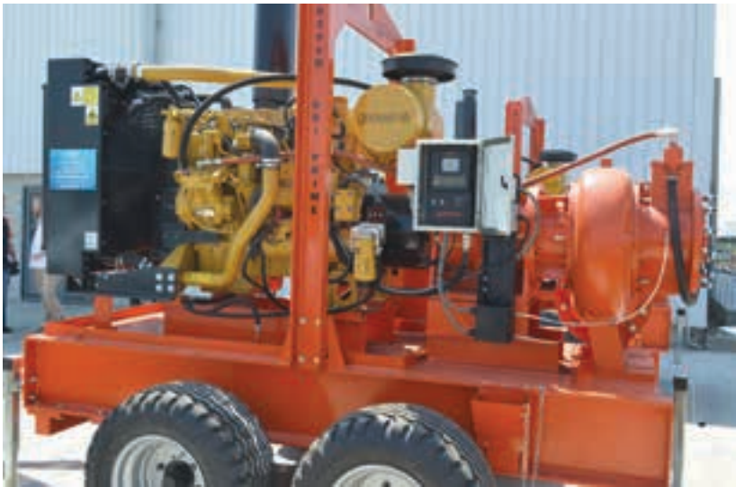
Godwin's CD range (contractor dewatering) is designed for general dewatering at high flows and medium heads. The engine is close-coupled to pump, so there are no alignment issues when it comes to maintenance.
