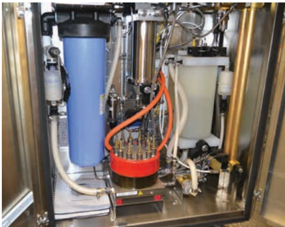
Above: HySA Infrastructure's largest hydrolyser at its NWU facility. The centre has the capacity to produce some 3.0 kg of H 2 per day from its solar system; equivalent to approximately 11.5 l of petrol per day.
