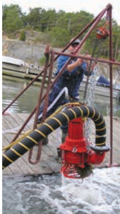
The Grindex Bravo submersible pump range is proving an efficient, cost effective alternate to vertical spindle pumps and is particularly well suited to the mining sector.
