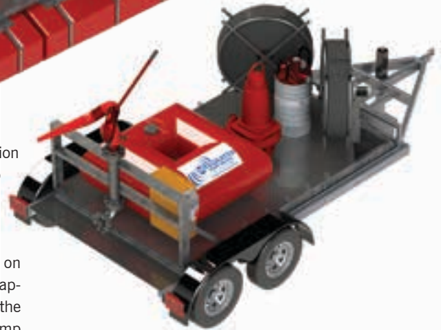
The Slurry Blaster is a cost effective cleaning tool that consists of a 37 kW feed pump with a float, a 22 kW Grindex slurry pump for the removal of the slurry, a 200 metre heavy duty layflat hose and an electric control panel. The unit is available on a pontoon (left), on a trailer (below) or with a support frame for manual use.
