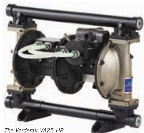
The Verderair VA25-HP (DA) is an FDA-approved AODD pump ideally suited to filter-press applications where the discharge pressure is higher than the available compressed air pressure.
