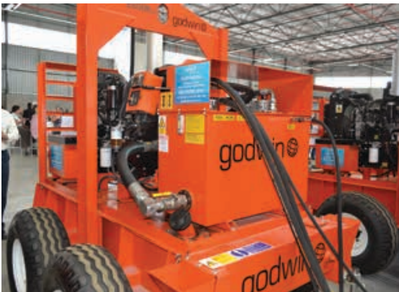
Xylem's Godwin Hydra pumps are hydraulic submersibles for use when suction lift of greater than 8.5 m is required. On these units, a diesel engine is used to drive a hydraulic power pack, which delivers biodegradable oil via hoses to a hydraulic submersible pump on the pond floor.
