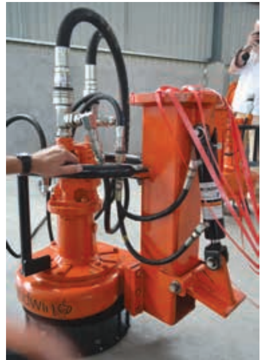
The Hydra's submersible pump head features a hydraulically activated slurry gate that can open in the event of clogging.
