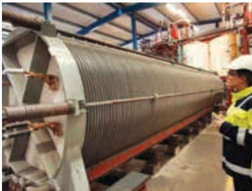
NEL Hydrogen has developed three standard models, which are modular in design and can be scaled up. These include the NEL A-150, providing between 50 and 150 Nm 3 /hour, the NEL A-300 that can generate up to 300 Nm 3 /hour and the NEL A-485 that can produce 485 Nm 3 /hour.
