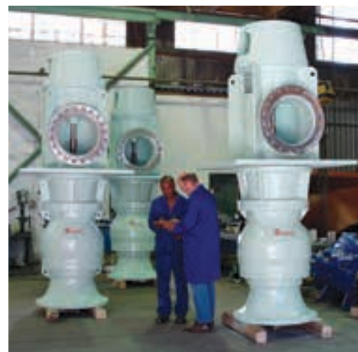
Vertical turbine pumps being manufactured in APE's Wadeville factory.
