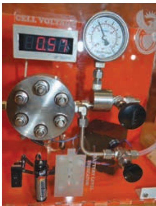
Above: HySA Infrastructure's largest hydrolyser at its NWU facility. The centre has the capacity to produce some 3.0 kg of H 2 per day from its solar system; equivalent to approximately 11.5 l of petrol per day.
