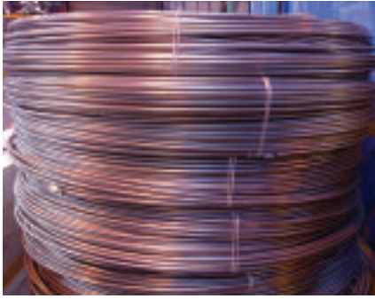
▲ The Energy Tubes product range includes coiled tubes up to 250m
