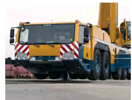
The Demag AC 300-6 is the smallest in the Demag range that can be outfitted with a luffing jib.
