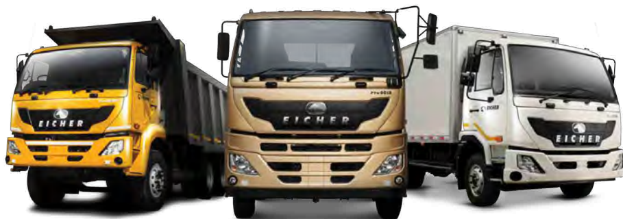
Three of the Pro series models for South Africa are the Pro 6025T, a 10 m 3 tipper; the Pro 6016, a 16 t GVM freight carrier; and the Pro 3000, an 8,5 t heavy duty offering for haulage.
