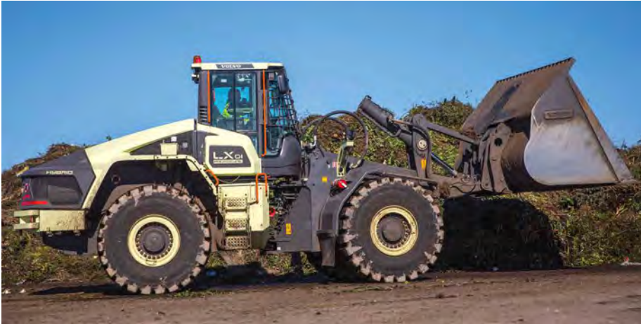
Volvo CE's LX1 prototype hybrid wheel loader performed hundreds of hours of real work in two applications at Waste Management facilities in California.
