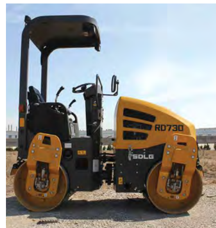
The RD730 is a 3 t capacity double drum asphalt compactor.
