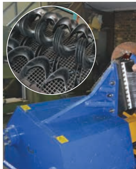
The company's new state-of-the-art fabricated/sectional flight manufacturing system starts with a CAD program, which generates the exact doughnut profile required for CNC laser cutting. Bruton Spiralflyte's continuous rolled flighting is widely used for screw conveyors or augers for moving cement, maize, coal, sugar cane and sand. These are loaded onto the pressing machine, which presses flights with identical pitch (inset).
