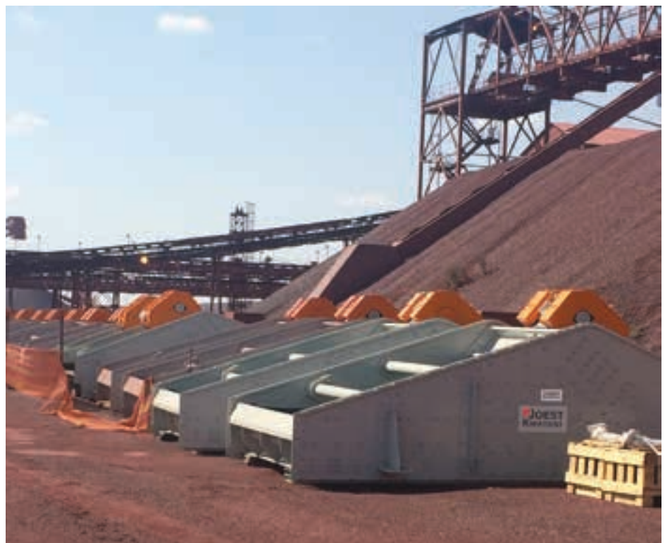
Joest Kwatani drain and rinse screens ready for installation into the mine’s cyclone plant.
