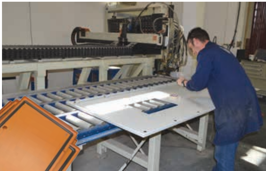
Above: WPP's CNC gasketing machine enables polyurethane foam gaskets to be fitted during the manufacturing process. Below: Enclosures in standard sizes and various
