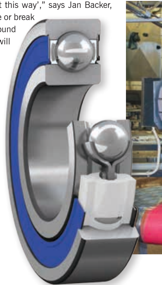
SKF’s new range of Food Line stainless steel deep groove ball bearings (VP311) meets two key requirements of the food industry: the seals are made from synthetic rubber compliant with US Food and Drug Administration (FDA) as well as European Community (EC) requirements and are coloured blue for optical detectability, should they be damaged; and they use high quality grease, suitable for food and beverage applications – registered as NSF category H1.
