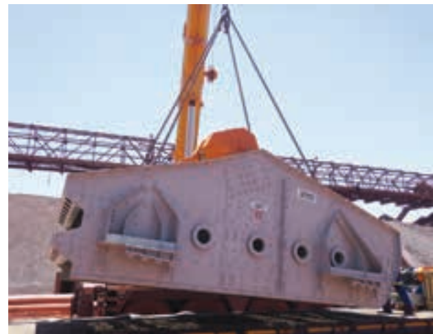
A Joest Kwatani double deck screen ready for installation at a washing and screening plant of the Kathu-based iron ore mine.
