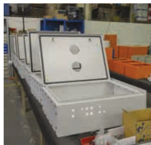
Above: WPP's CNC gasketing machine enables polyurethane foam gaskets to be fitted during the manufacturing process. Below: Enclosures in standard sizes and various
