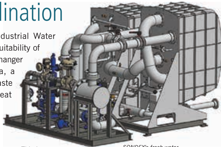
SONDEX's fresh water distillers utilise the waste heat from diesel engine jacket cooling water or other heat sources to produce pure drinkable water by evaporating seawater under high vacuum. This system produces up to 150 t of drinkable water per day.
