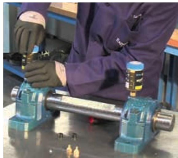
BMG has extended its range of lubrication products to include a single point lubricator, where the grease is pressurised by a gas generated unit to provide continuous, reliable, clean and precise lubrication.
