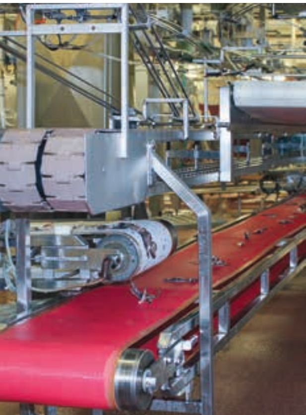
Above: The traditional wash down and relubrication cycle presents risks to both bearing service life and the environment. Left: In the food industry, for processing fish, for example, SKF has developed solutions that fulfil FDA and EC requirements. These bearings feature Re-lubrication free bearing technologies; high efficiency seals that keep lubricants in and contaminants out; and the use of corrosion resistant stainless steel materials.
