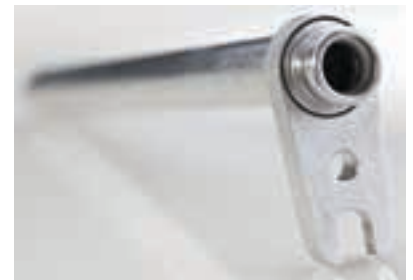
Axial tube forming with a spring follow-on tool can be used to attach an external component.
